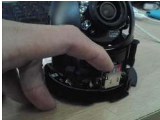
Gambar 5.1 Instalasi SD Card IP Camera
